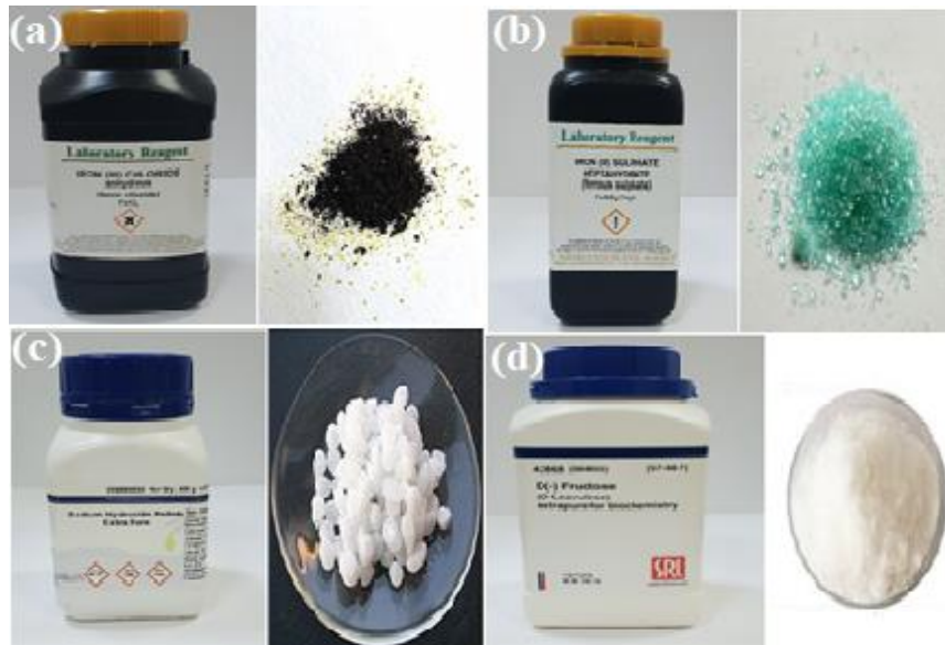
Fig. 1: Raw material used for the preparation of \text{Fe}_3\text{O}_4 , (a) Ferric chloride ( \text{FeCl}_3 ), (b) Ferris sulfate heptahydrate ( \text{FeSO}_4 \cdot 7\text{H}_2\text{O} ) (c) Sodium Hydroxide ( \text{NaCl} ) (d) D-fructose
