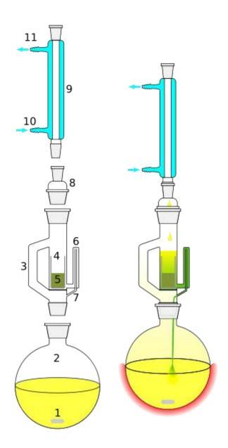
A schematic representation of a Soxhlet extractor
