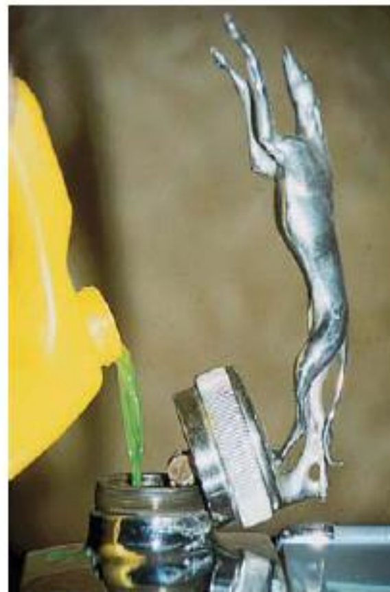
The addition of antifreeze lowers the freezing point of water in a car's radiator.
