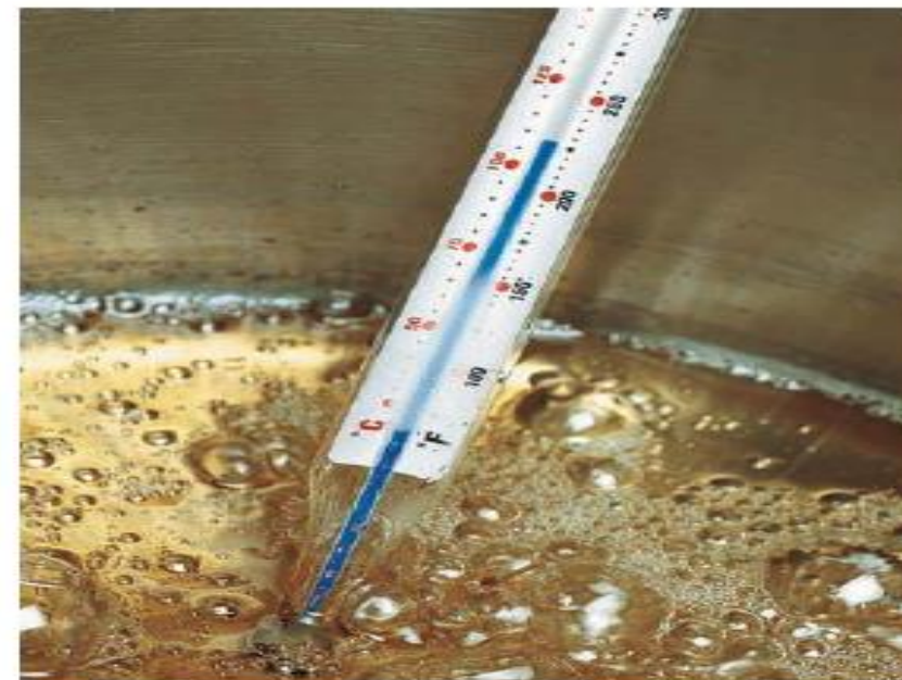
Sugar dissolved in water to make candy causes the boiling point to be elevated above 100°C.
